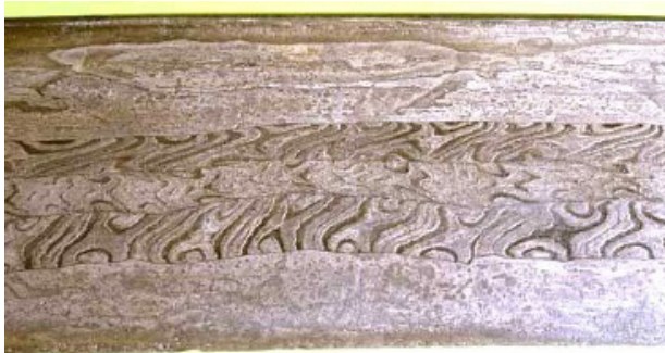
1 the layers of steel in a Saxon sword
